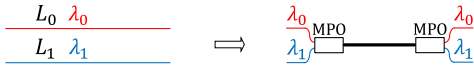
Fig. 3. Two vertically-aligned links can be implemented by a multi-fiber link containing two fibers.
